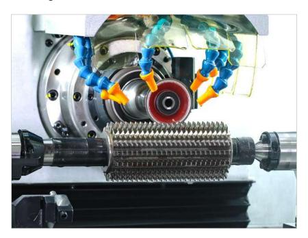
Precision, versatility, and shorter cycle time help users to reduce the regrinding cost of hobs and shaper cutters significantly. The hob inspection cycle on the machine checks the hob before removing it from the machine after regrinding.
